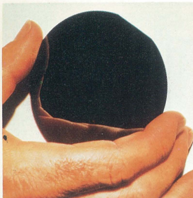
27 Section of a silicon crystal when first produced.
