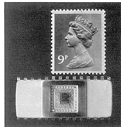
9 A modern microelectronic circuit, shown in the smallest square, can have more than 250,000 components.
